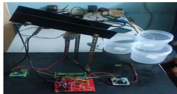
Fig. 9 Automatic Waste Segregator Prototype Set-up
