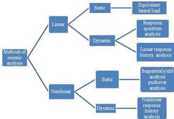
Figure 2. *Methods of seismic analysis*
