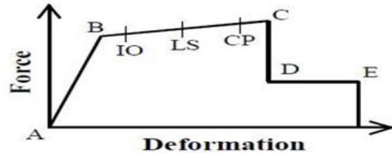
Figure 3. *Different Stages of Plastic Hinge Formation.*
