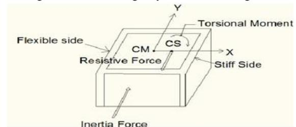
Figure 1. Generation of torsional moment in asymmetric structures
