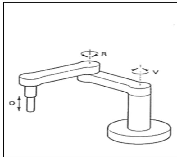
Figure 7 SCARA robots
