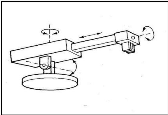
Figure 4 spherical workspace
