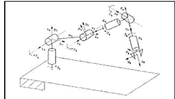
Figure 10. 6 link forward kinematics
