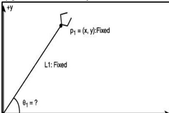
Figure 8 one link forward kinematics
