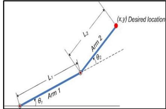
Figure 9 two link forward kinematics
