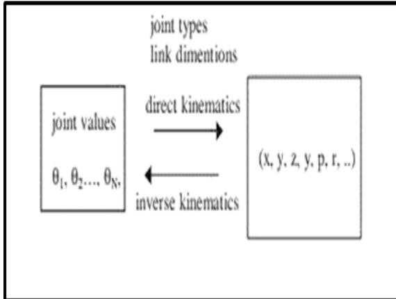
Figure 6 forward kinematics
