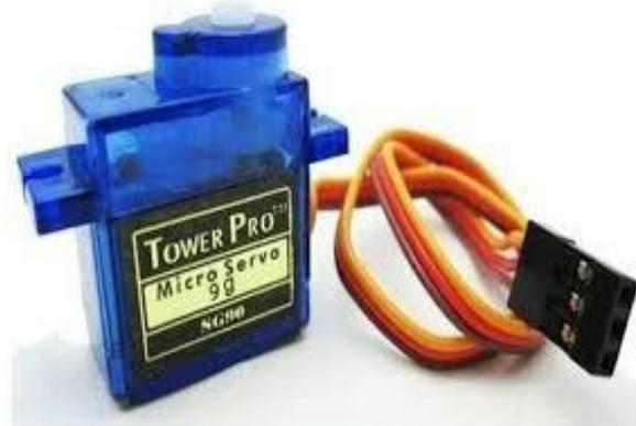
Figure: Servo Motor
