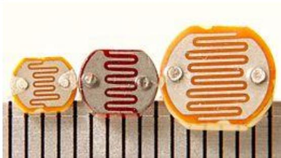
Figure: Photo Resistors
