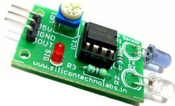
Figure 3: Infra-Red(IR) Sensors
