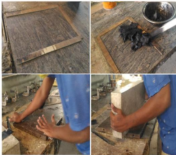
Figure 2 -Preparation of Mould and Curing of composite.
