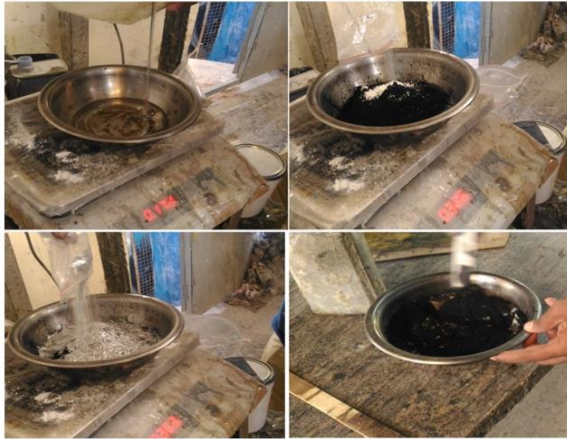
Figure 1- Weighing and mixing of the constituents. The mixture was poured in excess into a pre-prepared mould and subjected to compression moulding technique which is shown in Figure 2.
