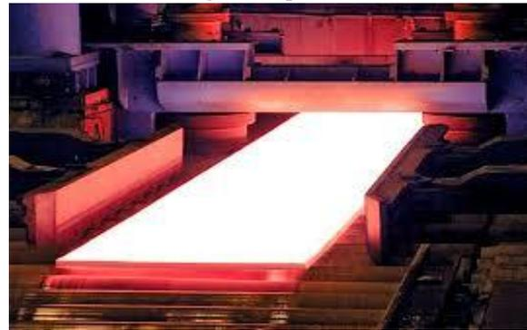
Fig -4 A hot plate exits the plate mill roller
