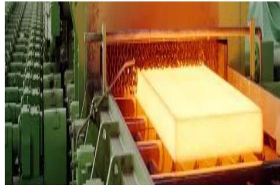
Fig -3 A hot steel slab exits the reheating furnace before moving to the plate mill section.
