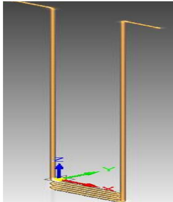
Fig 4: Experimental earth tube heat exchanger
