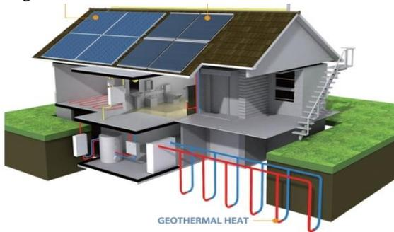
Fig 3: Closed type earth tube heat exchanger [10]
