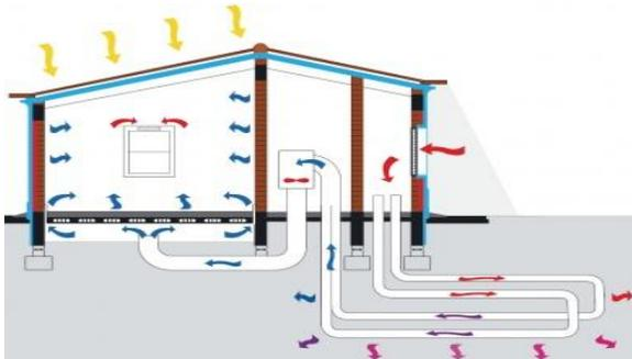
Fig 2: Open type earth tube heat exchanger [8]
