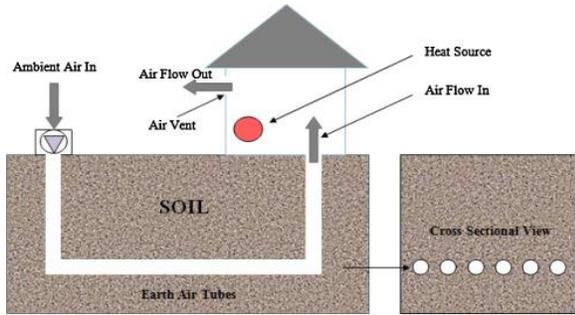
Fig -1: Earth tube heat exchanger [9]
