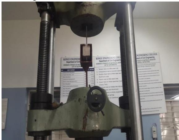
“Fig. 3” Pull-out test set-up
