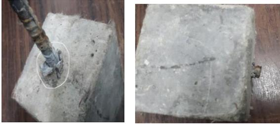
“Fig. 6 The crack development on four faces in ECC specimen
