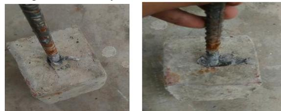
“Fig. 5 Pull-out test failure and crack development in ECC specimen
