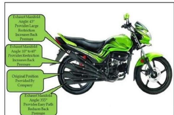
Fig. 2. Effect of change of exhaust slant on back pressure
