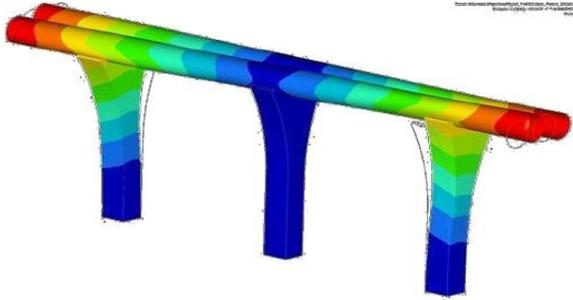
Fig. VIII. First mode shape of Hyperloop at 2.71Hz (magnified x1500)
