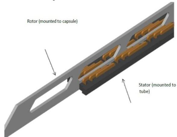
Fig. V. Rotor and Stator 3D Diagram
