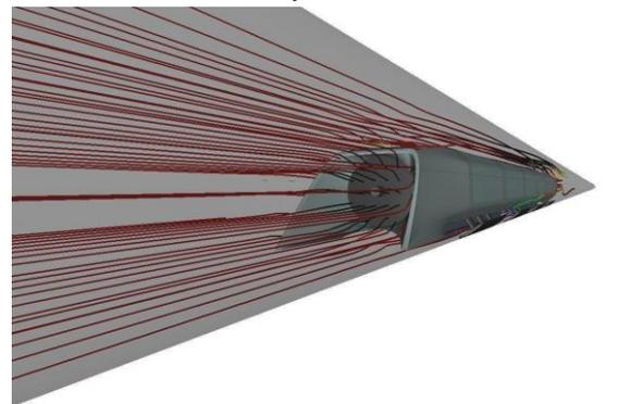
Fig. IV. Streamlines for capsule traveling at high subsonic velocities inside Hyperloop.
