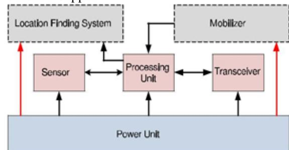
FIG 1. The architecture of the sensor node
