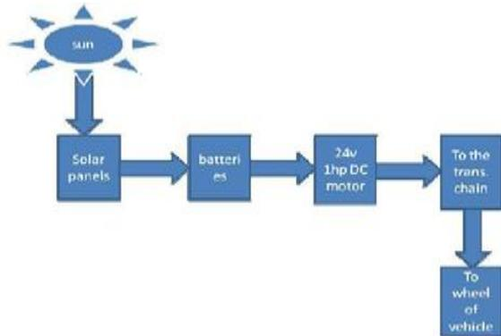
Fig.2 Basic block Diagram Representation of Solar vehicle.
