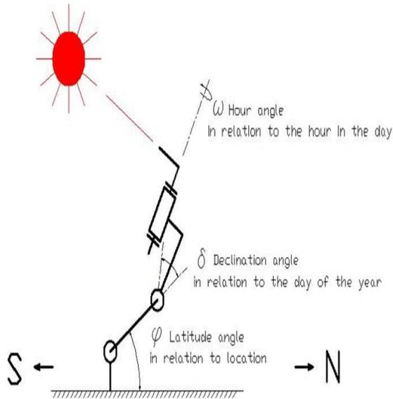
Figure 4: Kinematic chain for solar trajectory
