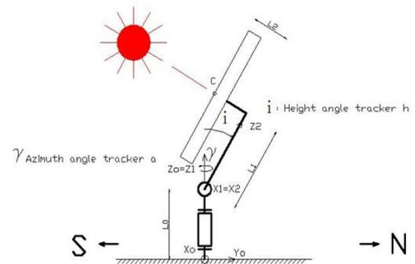
Figure 3: The Altazimuth tracker
