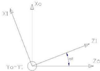
Figure 1: Rotation around y axis
