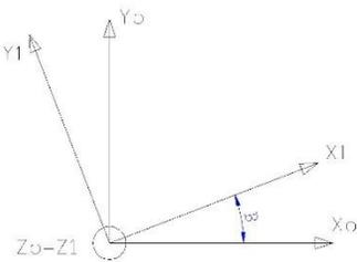
Figure 2: Rotation around z axis
