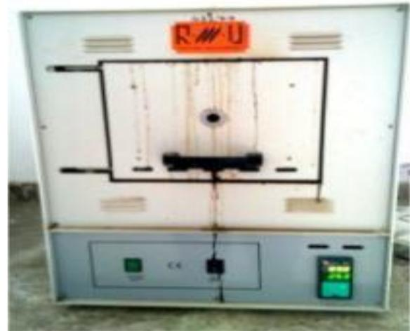
Fire resistance test was done to find out effects of fire on the properties of AAC. Test was done on 50x50x50 mm cubes at six different temperatures. These temperatures were fixed to be 100° 300°C. 500°C, 700°C, 900°C and 1000°C, and were on the electrical muffle furnace. Three AAC samples were tested for each temperature.
