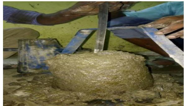
Figure 2. SLUMP CONE TEST
