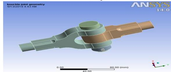
Fig.2.1) 3D Geometry of knuckle joint
