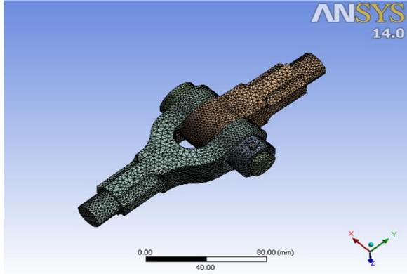
Fig.3.1) Meshing of knuckle joint made
