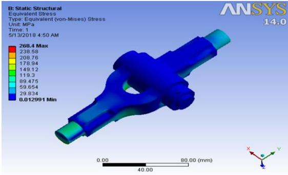
Fig.5.1) Equivalent stress for grey cast iron and structural steel
