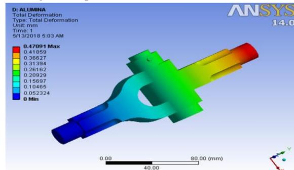
Fig.5.6) Total Deformation for Alumina (Saffil)
