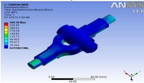
Fig.5.3) Equivalent stress for Carbon fibre
