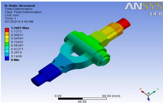
Fig.5.2) Total Deformation for grey cast iron and structural steel
