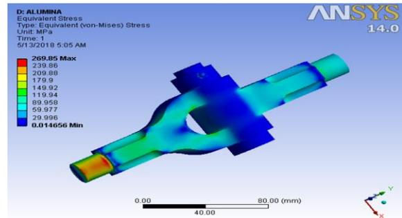
Fig.5.5) Equivalent stress for Alumina (Saffil)
