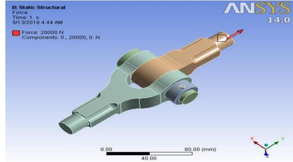
Fig.4.2) Tensile force at Eye end
