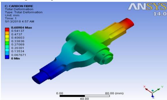
Fig.5.4) Total Deformation for Carbon fibre
