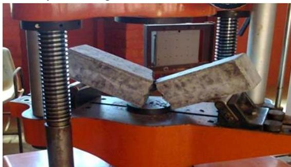
Figure.5.Flexural strength test
