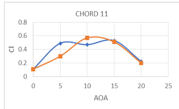
Figure 6: Co-efficient of Lift for Normal and spanwise blowing on sweptback wing. The Figure 6 which is similar to C l versus angle of attack graph of chord 12.5. Here both C l and stalling angle are increasing for spanwise blowing. This shows that leading-edge vortex breakdown is reduced and boundary layer separation is delayed than without spanwise blowing.
