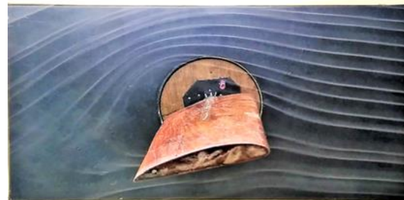
Figure 3. Smoke flow visualization of wing with spanwise blowing
