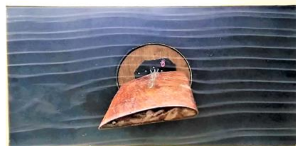
Figure 2. Smoke flow over the wing without spanwise blowing
