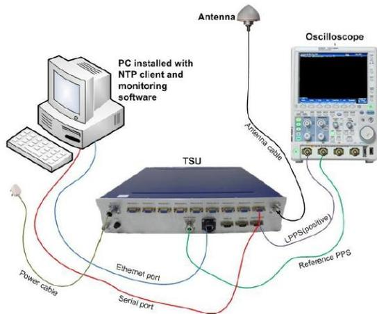
Fig 5: System Set up diagram
