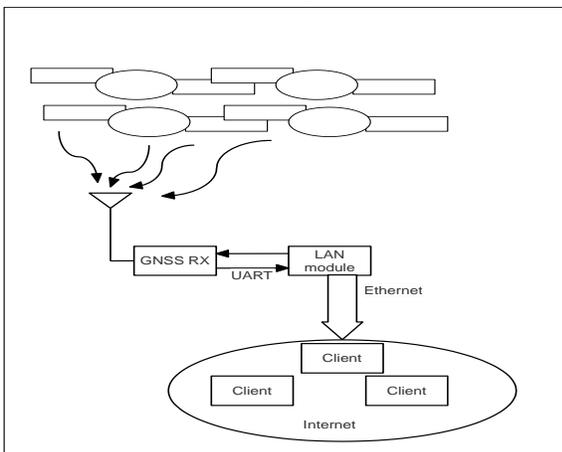
Fig 1: System architecture of GNSS based NTP
