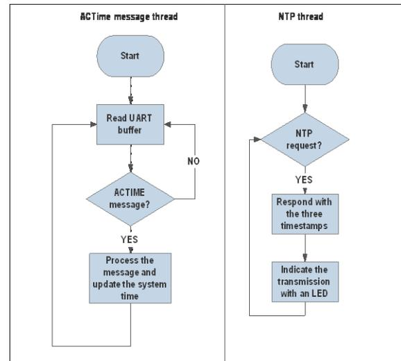
Fig 2: ACTime message and NTP thread
