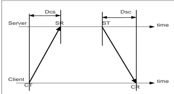
Fig 2 : Time synchronizing using NTP
