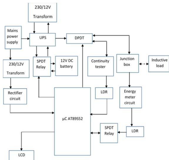
Fig.2.1: Block diagram of power saving smart inverter
