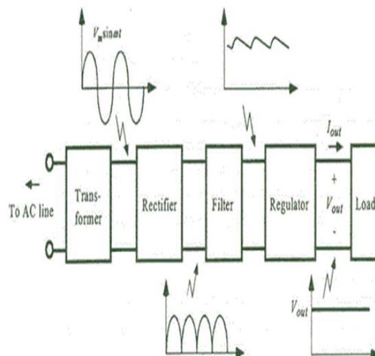
Fig.3.1: Block diagram of regulated power supply
