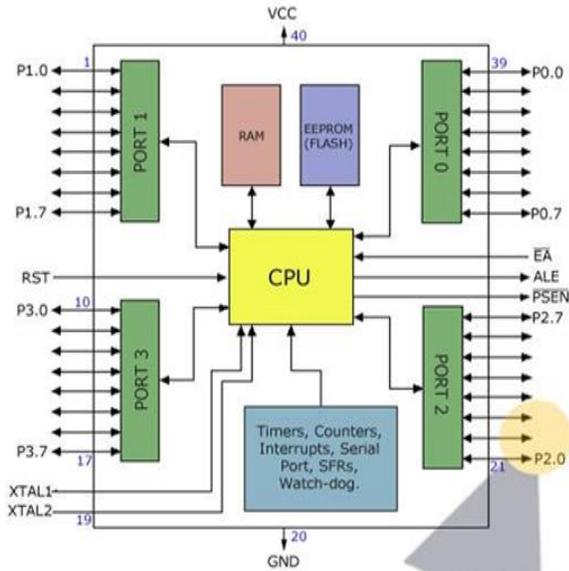
Fig.3.4: Block diagram of microcontroller 8051
