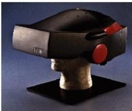
**Figure 1.11 Head Mounted Display**
