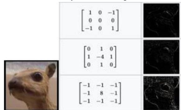
FIGURE 4. Original image (left) filtered by example edge detection kernels
