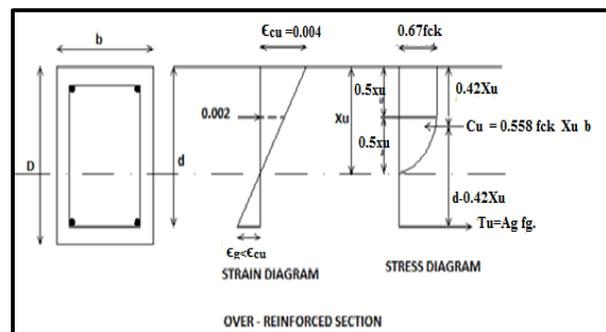
Diameter of Bars = 10 mm  $\phi$ , Tensile stress ( $f_{gu}$ ) = 600 MPa , Modulus of elasticity ( $E_g$ ) = 50 GPa,  $f_{ck}$  = 30 MPa ,  $b$  = 150 mm ,  $D$  = 150 mm ,  $d$  = 130mm ,  $L$  = 700 mm.
