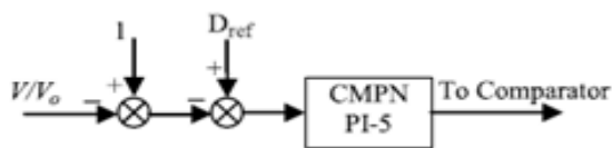
Fig 3. Control of the DC-DC converter.
