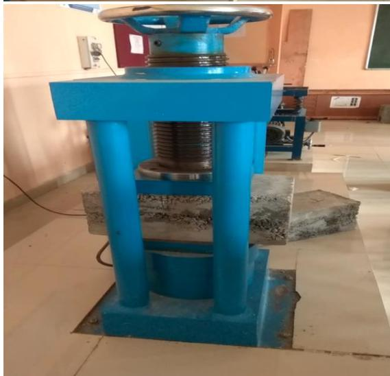
Fig. Testing of block under CTM machine"
