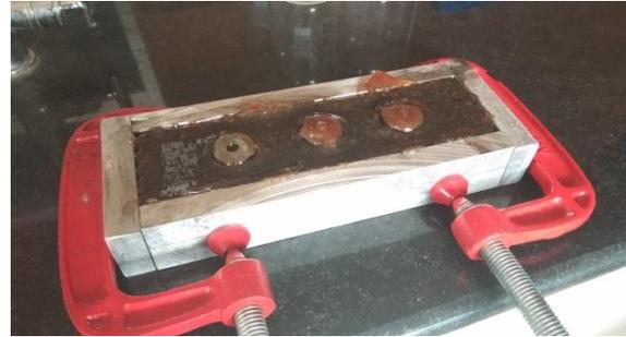
Fig. Melted PET plastic in the mould
