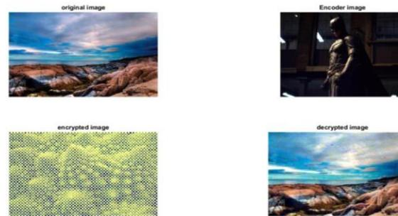
Fig. 4. Encryption and decryption process with reference image.
