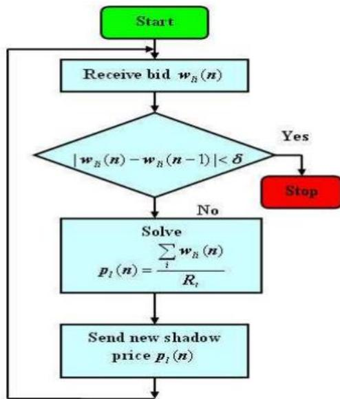
Figure 3.2: eNodeB Algorithm of Joint Carrier Aggregation
