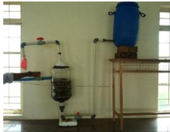
Fig: 3: UASB Reactor Before Production of Biogas
