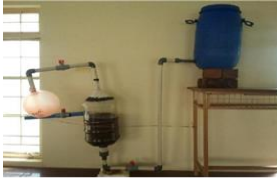
Fig: 4: UASB Reactor After Production Of Biogas The chemical characteristics of tanner waste water are illustrated .The tests are carried out before the treatment.
