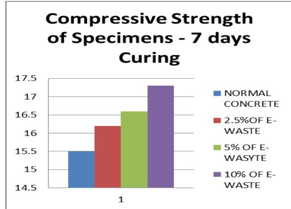
Figure 1: Compressive Strength of Specimens -& 7Days Curing Time
