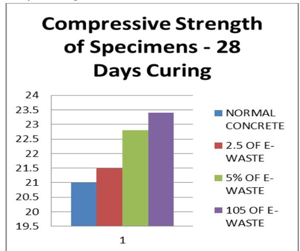
Figure 1: Compressive Strength of Specimens -& 28Days Curing Time
