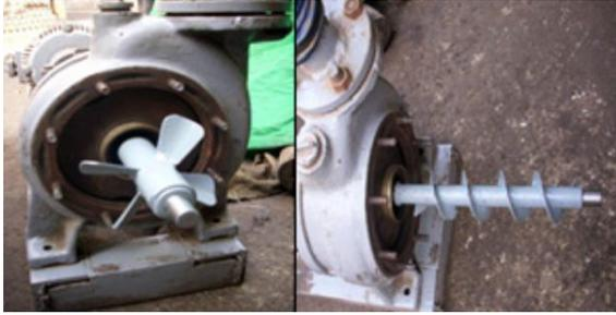
Fig. 2.2 Axial and Helical inducers in conjunction with the tested pump, respectively
