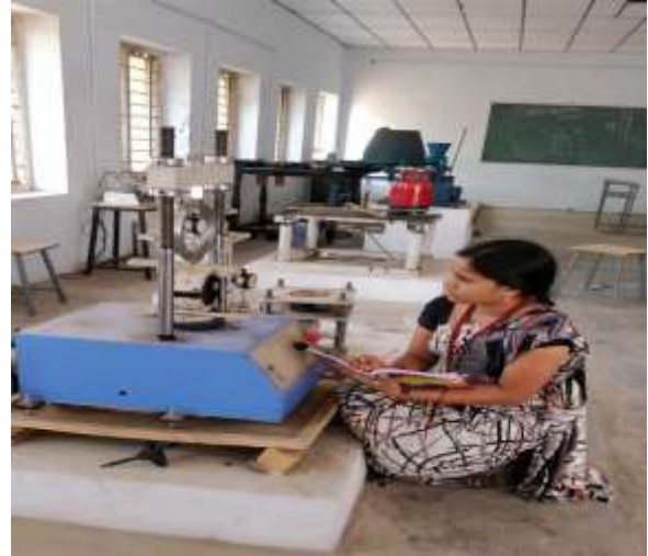
Figure 5: Marshall Stability Test apparatus
