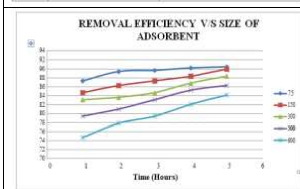
Fig. 4.4 Effect of adsorbent size on the removal efficiency of LAS ions
