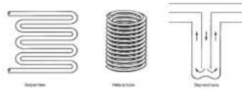
Figure 1.2 Additional tube configurations used in shell-and-tube exchangers
