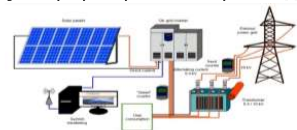
Figure 3: grid connected Solar System
