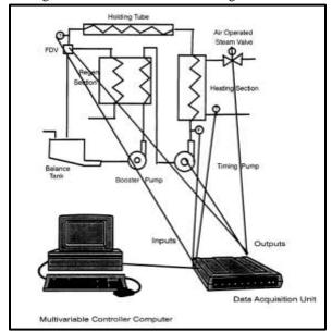
Figure 1.Schematic Diagram of HTST pasteurization system with computer control.
