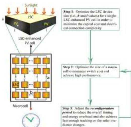
Fig. 8. The overall flow of the proposed LSC-based PV array reconfiguration and optimization.
