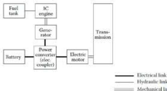
PARALLEL PHEV-both the engine and electric motor are mechanically connected to the wheels, and both propel the vehicle under most driving conditions. Electric only operation usually occurs at Lower speeds.
