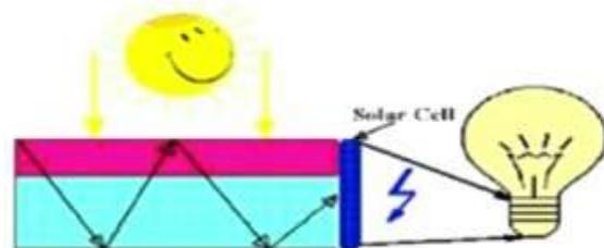
In current LSC when the sunlight hits the top part of the device the sun's energy is transformed into the dye molecules causing the electrons in the dye molecules to excite into higher energy level .when the electrons falls back to lower energy level the dye molecules release that energy into plastic sheets on
