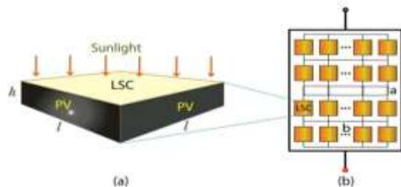
It's better to make LSC enhanced pv cell a square top surface so that solar irradiance concentrated on four sides are identical.
