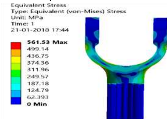
Figure 7. Gearbox side Universal joint
