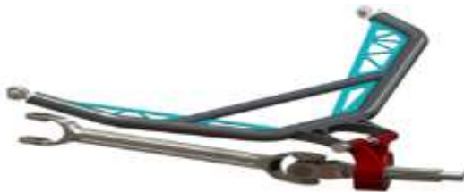
Figure 3. Parallelogram Suspension Geometry The geometry is optimized to yield a roll centre of 16" and zero camber and toe change. It is in
