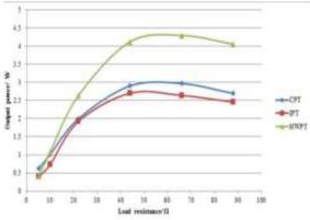
Green represents the output power of HWPT. Blue is the output power of CPT and Red is for IPT. The output power of HWPT is higher than IPT and CPT.
