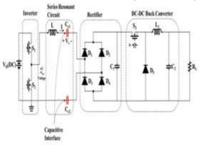
Compared to IPT, CPT has advantages such as reduced cost and weight .CPT has the ability to transfer energy through metal. Therefore it can be used for wireless charging of smartphone.
