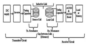
This WPT charging gives a far lower risk of electrical shock because it is galvanically isolated. In WPT the coupling coefficients reducs when the transfer distance increases.
