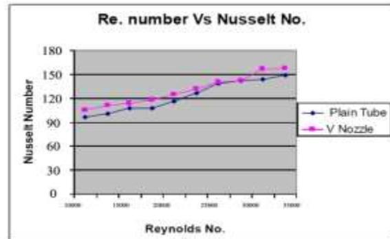
The graph shows the relations between Reynolds no and nussult no. the nussult no increases with the increase in the Reynolds no. and the Reynolds no increases in the v-nozzle.
