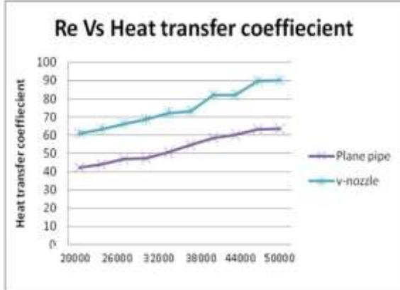
The graph shows the relations between Reynolds no and heat transfer coefficient. The heat transfer coefficient increases with the increase in the Reynolds no. and the friction factor increases in the v-nozzle.
