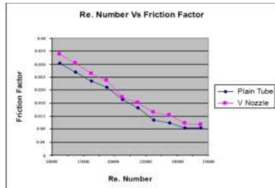
The graph shows the relations between Reynolds no and friction factor. the friction factor reduces with the
