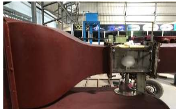
Figure 1. Contraction cone and test section.
