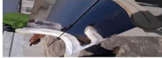
Fig 9. Copper pipe placed at focus.
