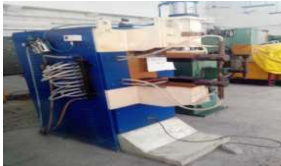
Fig.2 Resistance spot welding machine
