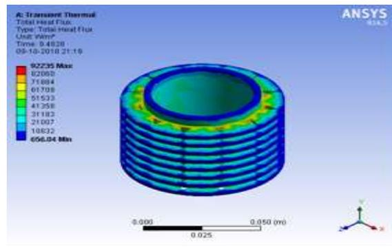
Fig 6 Total heat flux contour of cylindrical block having Aluminium alloy circular fin with triangular hole
