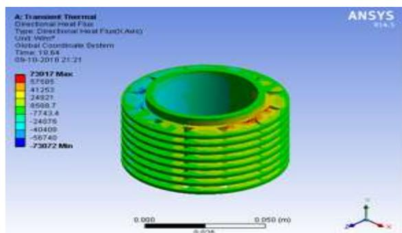
Fig 7 Directional heat flux contour of cylindrical block having Aluminium alloy circular fin with triangular hole
