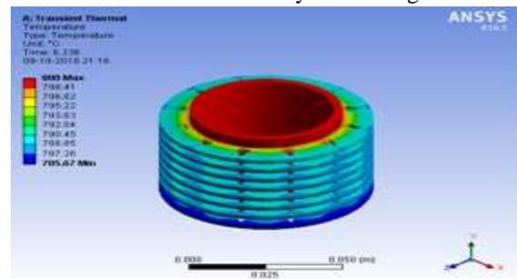
Fig 5 Temperature contour of cylindrical block having Aluminium alloy circular fin with triangular hole
