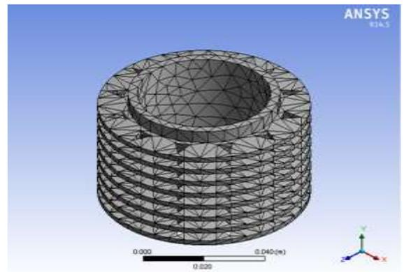
Fig 3 The meshing of cylindrical block having circular fins with triangular holes.
