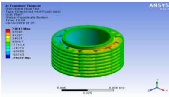
Fig 10 Directional Heat flux contour of cylindrical block having Magnesium alloy circular fin with triangular hole
