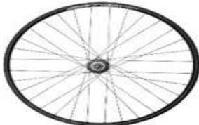
Wheel is used to carry the whole assembly and move machine from one place to another by rotary motion of it. A bicycle wheel is a wheel, most commonly a wire wheel, designed for a bicycle. Bicycle wheel is designed to fit into the frame and fork via drop outs, and hold bicycle tire. A typical modern wheel has a metal hub, wire tension spokes and a metal or carbon fiber rim which holds a pneumatic rubber tire. We use a tubeless tire wheel.
