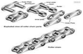
The chain is made of steel which is used to transmit power from gear sprocket to pinion sprocket, and it has a no sleep.
