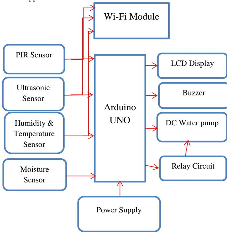
Fig3.1 Block diagram of smart agriculture system
