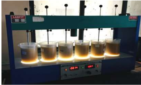
Figure- 2 : Fenton process with coagulation
