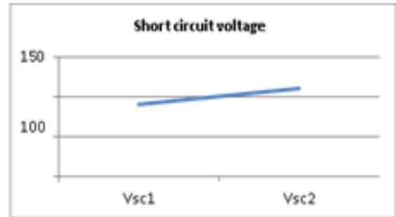
Fig 1: Short circuit voltage of healthy (Vsc1) & core deformed transformer (Vsc2)
