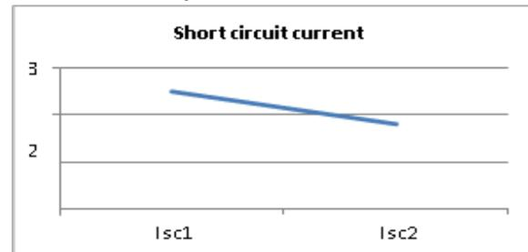
Fig 2: Short circuit current of healthy (Isc1) & core deformed transformer (Isc2)
