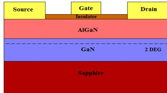
Fig 1: Cross section view of HEMT
