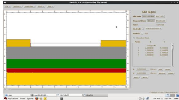
Fig 13: Etching of the SiO2
