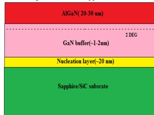
Fig 2: Layered structure of AlGaN/GaN HEMT
