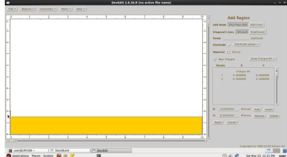
Fig 5: Defining a sapphire substrate
