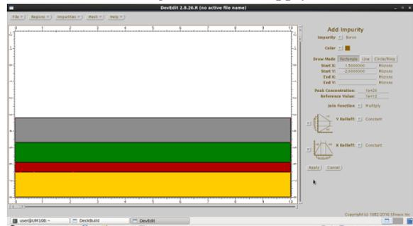
Fig 8: Deposition of AlGaIn layer
