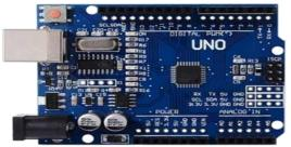
The output of the comparator is given to the digital pin 8. The Arduino is programmed in such a way that whenever there is an input high at the digital pin 8, then the TX pin i.e. pin1 gets activated and the transmitter Bluetooth module which is acting as master transmits the signal to the receiver side Bluetooth module.
