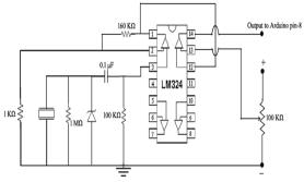
Components in triggering circuit: Piezo electric transducer:
