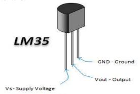
LM35 has three pinouts which are:
